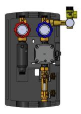
Pump group is a device that ensures and regulates the circulation of the solar fluid between the solar collectors and the tank. The group consists of a circulating pump as well as control and measuring devices. It can be used both for flat solar collectors and for vacuum collectors. The advantage of the double pump group is that it enables controlling the temperature of the solar system heating medium supply and the return.
