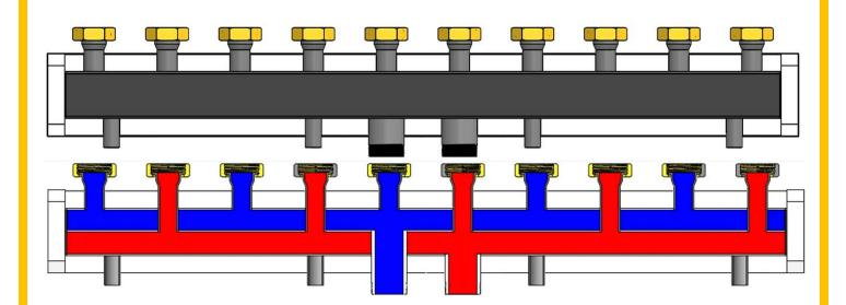
The distributor is designed for central heating installations of 150 kW with the possibility of connecting 5 pump groups. Made of steel, it is enclosed in EPS insulation and powder-coated steel sheet to reduce heat loss. It is used to facilitate the installation of mixing and pumping groups. Enables reducing the number of installation devices. This saves space, time and installation costs. Brackets, screws, wall plugs and washers for wall mounting are included.
