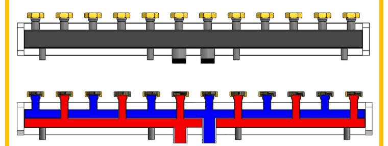
The distributor is designed for central heating installations of 150 kW with the possibility of connecting 6 pump groups. Made of steel, it is enclosed in EPS insulation and powder-coated steel sheet to reduce heat loss. It is used to facilitate the installation of mixing and pumping groups. Enables reducing the number of installation devices. This saves space, time and installation costs. Brackets, screws, wall plugs and washers for wall mounting are included.
