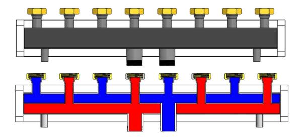
The distributor is designed for central heating installations of 150 kW with the possibility of connecting 4 pump groups. Made of steel, it is enclosed in EPS insulation and powder-coated steel sheet to reduce heat loss. It is used to facilitate the installation of mixing and pumping groups. Enables reducing the number of installation devices. This saves space, time and installation costs. Brackets, screws, wall plugs and washers for wall mounting are included.
