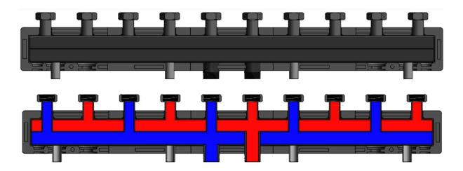
The distributor is designed for central heating installations of 120 kW with the possibility of connecting 5 pump groups. Made of steel, it is enclosed in expanded polypropylene insulation to reduce heat loss. It is used to facilitate the installation of mixing and pumping groups .Enables reducing the number of installation devices. This saves space, time and installation costs. Brackets, screws, wall plugs and washers for wall mounting are included.
