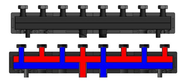
The distributor is designed for central heating installations of 120 kW with the possibility of connecting 4 pump groups. Made of steel, it is enclosed in expanded polypropylene insulation to reduce heat loss. It is used to facilitate the installation of mixing and pumping groups. Enables reducing the number of installation devices. This saves space, time and installation costs. Brackets, screws, wall plugs and washers for wall mounting are included.
