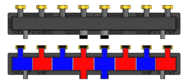
The distributor is designed for central heating installations of 120 kW with the possibility of connecting 4 pump groups. Made of steel, it is enclosed in expanded polypropylene insulation to reduce heat loss. It is used to facilitate the installation of mixing and pumping groups. Enables reducing the number of installation devices. This saves space, time and installation costs. Brackets, screws, wall plugs and washers for wall mounting are included.
