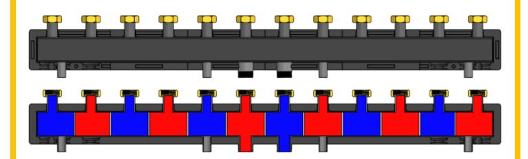
The distributor is designed for central heating installations of 120 kW with the possibility of connecting 6 pump groups. Made of steel, it is enclosed in expanded polypropylene insulation to reduce heat loss. It is used to facilitate the installation of mixing and pumping groups. Enables reducing the number of installation devices. This saves space, time and installation costs. Brackets, screws, wall plugs and washers for wall mounting are included.
